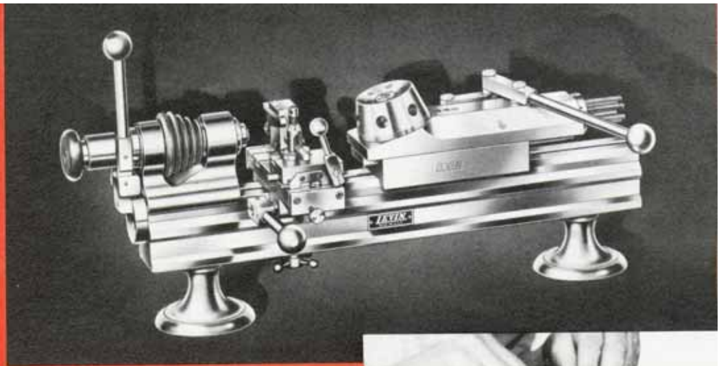
LATHE WITH COLLET CLOSER, CROSS SLIDE & POSITION TURRET 1 1/2" BEEF
