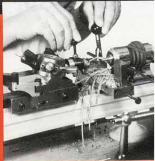
LATHE WITH COLLET CLOSER, CROSS SLIDE & POSITION TURRET 1 1/2" BEEF
