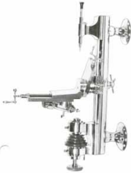
Lathe with Wheel Cutter and Milling Tool also Plain Tailstock.
