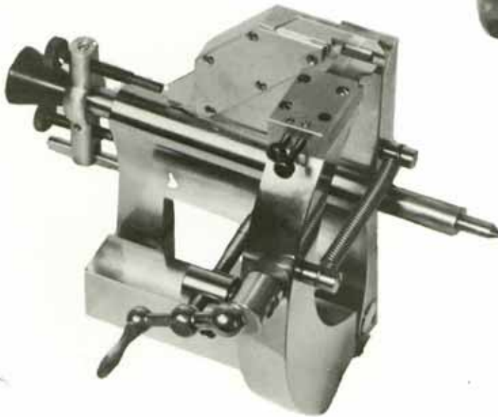
Elect Jeweling Rest with Caliper, Depthing Device and Cross Feed Screw. For cutting outside and inside diameters for jewels or settings. Depthing device is for gauging depth of recess for setting or jewel. Cross Feed Screw is for turning and facing up work. Cat. No. 3038.
