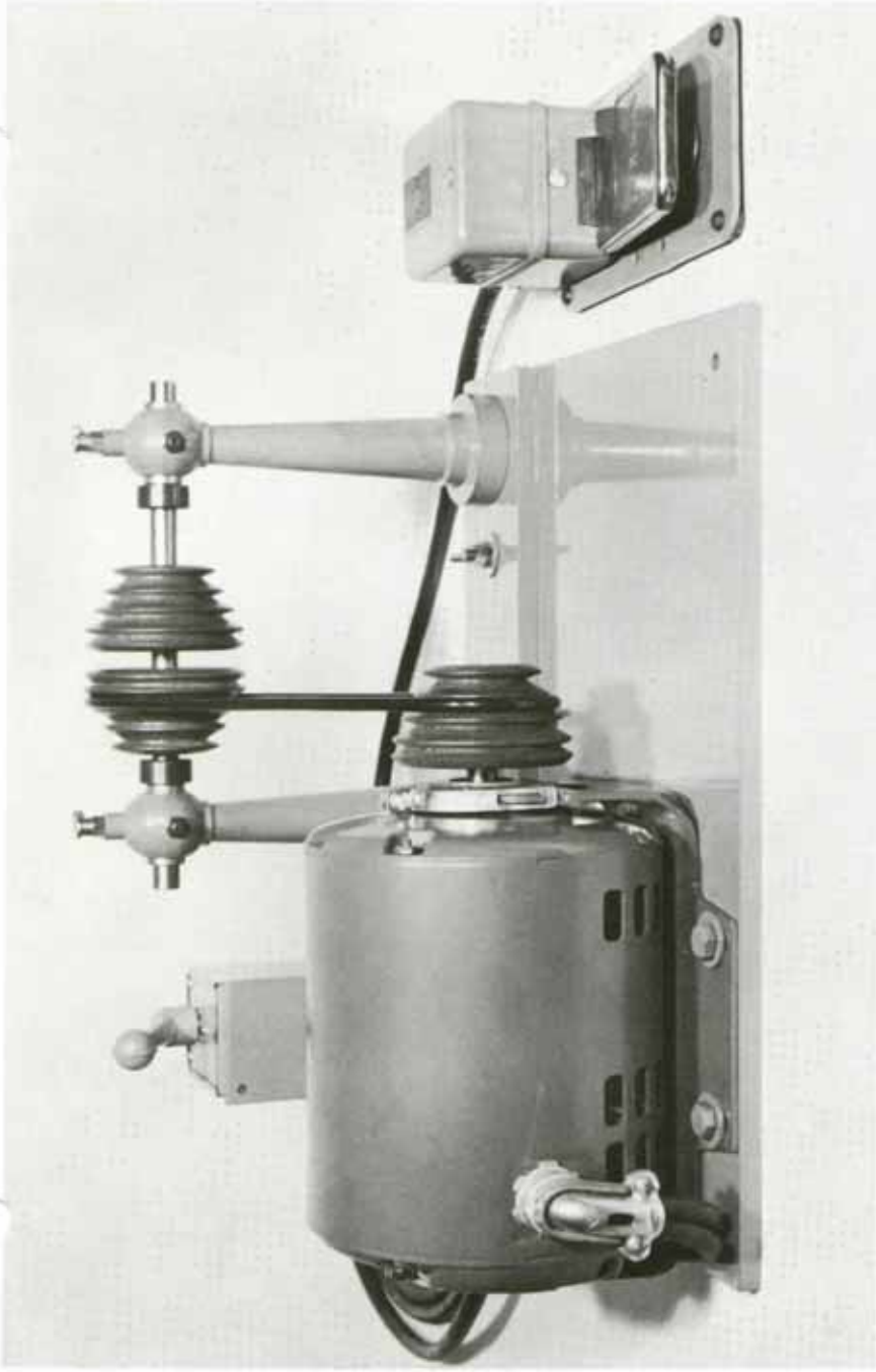
COMPLETE MOTOR DRIVE UNIT Motor Unit, 15" x 11" complete with \frac{1}{2} HP, 60 cycle, 1 phase Motor or \frac{1}{4} HP, 60 cycle, 1 phase Motor, with Cutter-Hammer Drum Reverse Switch and Furnas Foot Switch, Countershaft and Pulleys. Wired and ready to plug in. Speeds obtainable are from 400 to 2800 RPM in 12 steps of approximately 200 RPM from Motor to Countershaft to Lathe. Unit sets on top of bench and two screws only are needed to hold unit on bench. Pt. No. 10230 and 10240. \frac{1}{2} HP Motor for MAGNUS, D.W.W. and D-LARGE Lathes. \frac{1}{4} HP Motor for ELECT and MODEL 750 Lathes.
