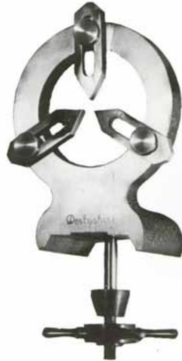
Back Rest w/shoe bolt, nut, and washer
