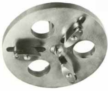
Universal Face Plate mounted on chuck stem.
