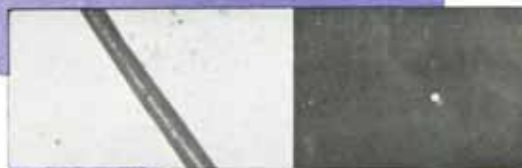
Human hair shown on left, hole drilled on right. Both are magnified 108 times.
